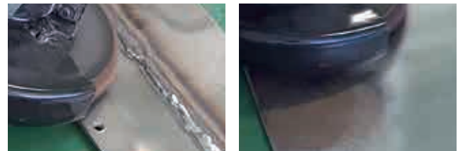
Removing blue weld discoloration Removing Rust
